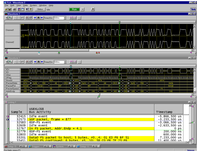
Left: Acquisition of USB device enumeration bus activity shown in three related listing display windows: basic-level bus event and packet display (with start-of-transaction packets highlighted, and display of EOP and Idle events as well as SOF packets suppressed) (top); transaction-level display (with setup transactions highlighted) (middle); control transfer-level display (bottom). Right: Multi-window display of DSO capture of full-speed D+ and D- signals (top), along with low-level logical view of the same signaling (middle), plus high-level event/packet protocol interpretation (bottom).
